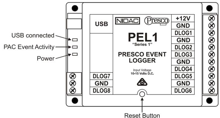
The **Power LED** indicates that the PEL has power and is working. The first time it is powered up this led will flash until the memory and clock have been initialised.
