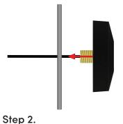
Remove the nut from the thread. Peel the protective layer from the adhesive on the back of the antenna. Push the thread through the hole in your casing.
